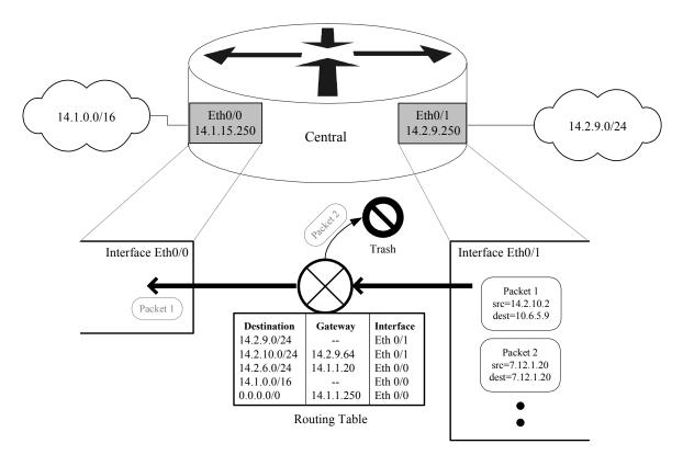
Figure 4-7: IP Unicast RFP Verification
