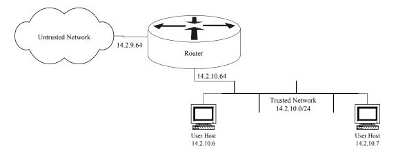
Figure 5-1: A Simple Router Firewall
