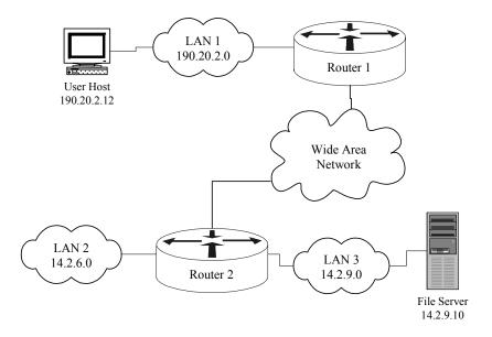
Figure 1-1 – A Simple Network with Two Routers
