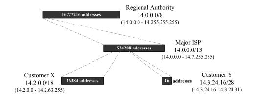
Figure 2-4: Hierarchical IP Address Range Assignment under CIDR
