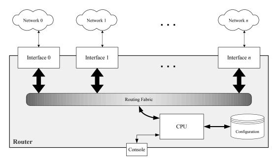
Figure 2-5: A Notional Router's Hardware Structure
