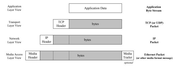
Figure 2-3: Wrapping Lower Level Headers around Data
