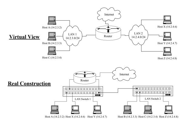
Figure 7-1: Virtual LAN Switching
