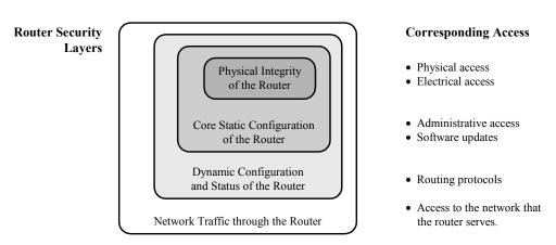
Figure 3-8: Layered View of Router Security
