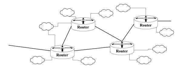
Figure 3-3: Backbone Routers Connect Many Networks
