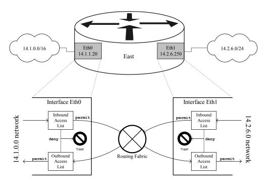
Figure 4-2: Conceptual Model for Access Lists on Interfaces
