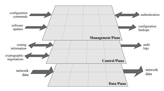
Figure 3-1: Three-Plane Conceptual Model for a Router
