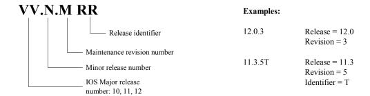
Figure 8-1 – Cisco IOS Release Naming
