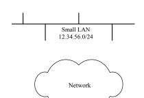
A local-area network (LAN) segment, such as an Ethernet, is represented by a horizontal or vertical bus, with several connections.
