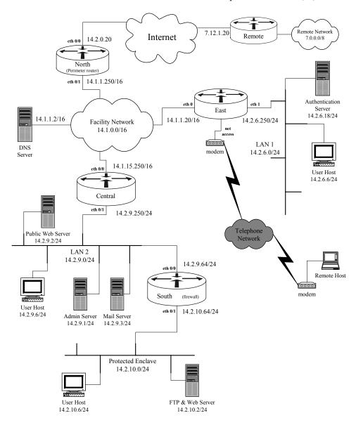
Figure 4-1: Example Network Architecture
