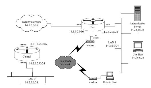
Figure 4-13: Router East in the Network
