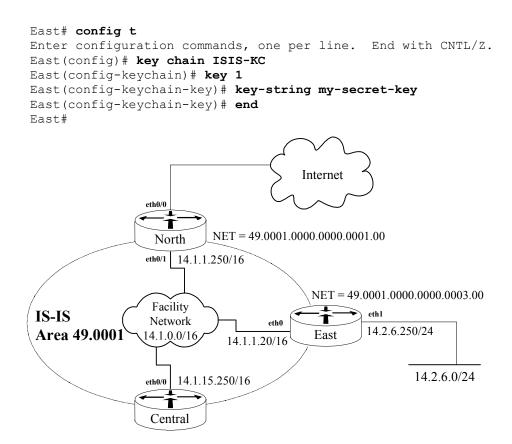
Figure 4-5: An Example Routing Architecture
