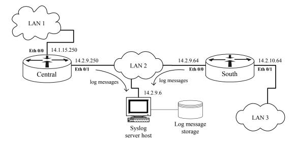
Figure 4-9: A Small Syslog Configuration
