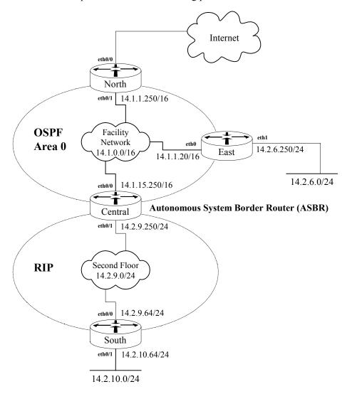
Figure 4-3: An Example Routing Architecture
