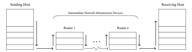
Figure 2-2: Moving Data through Protocol Stacks
